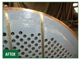
Tube sheet resurfaced using **Novocoat EP5700 Ceramic Paste.**
